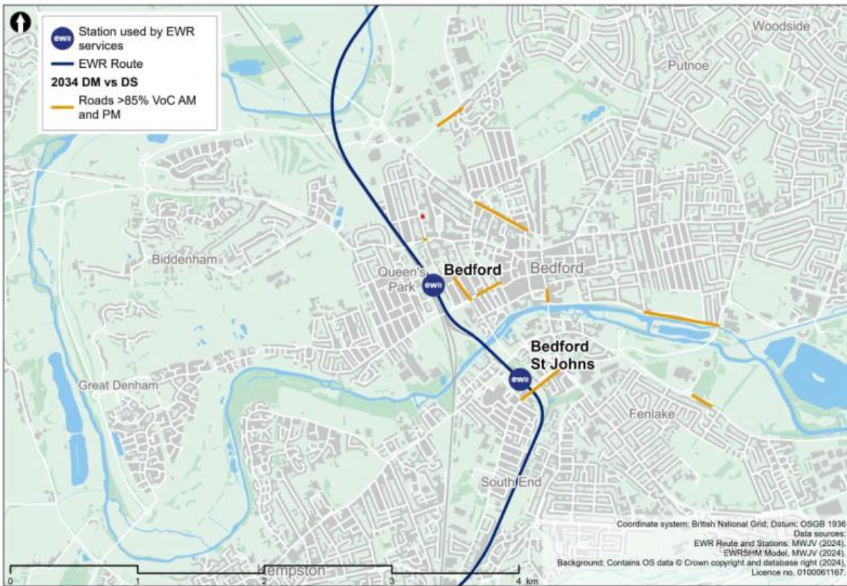
Figure 3.6: Additional Links with Forecast Volume-Capacity Ratio \geq 85\% in 2034 With Scheme Scenario (TUR Figure 48)
